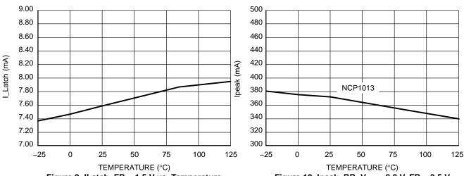
Figure 9. ILatch, FB = 1.5 V vs. Temperature
