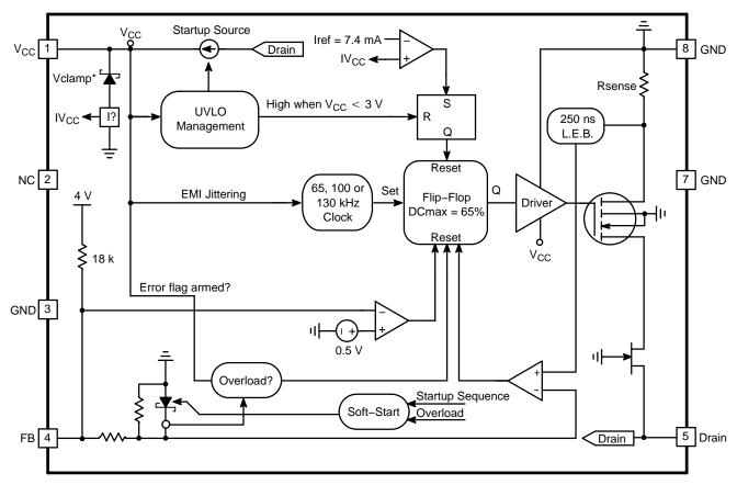
\*Vclamp = VCC<sub>OFF</sub> + 200 mV (8.7 V Typical)
