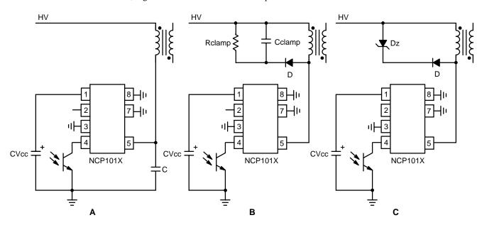
Figure 27. Different Options to Clamp the Leakage Spike
