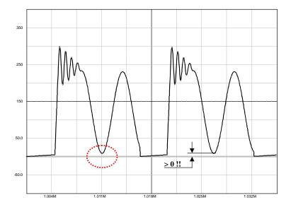
Figure 26. The Drain-Source Wave Shall Always be Positive . . .
