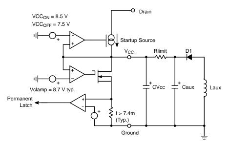
Figure 18. A more detailed view of the NCP101X offers better insight on how to properly wire an auxiliary winding.
