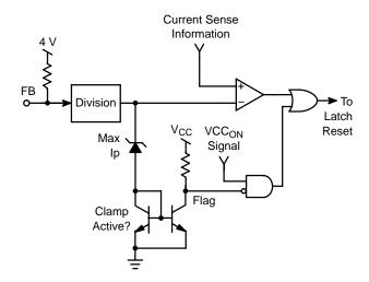
Figure 15. Simplified NCP101X Short-Circuit Detection Circuitry
