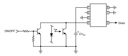
Figure 23. A non-latching shutdown where pulses are stopped as long as the NPN is biased.
