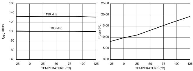
Figure 11. Frequency vs. Temperature
