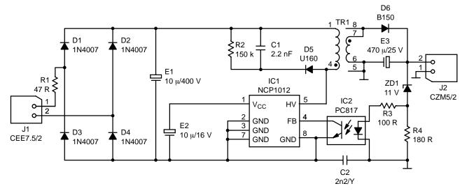
Figure 28. An NCP1012-Based Flyback Converter Delivering 6.5 W
