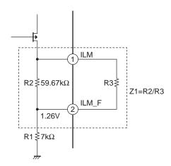
The ILM\_F voltage is determined by the internal band gap voltage of the IC (typ = 1.26V).
