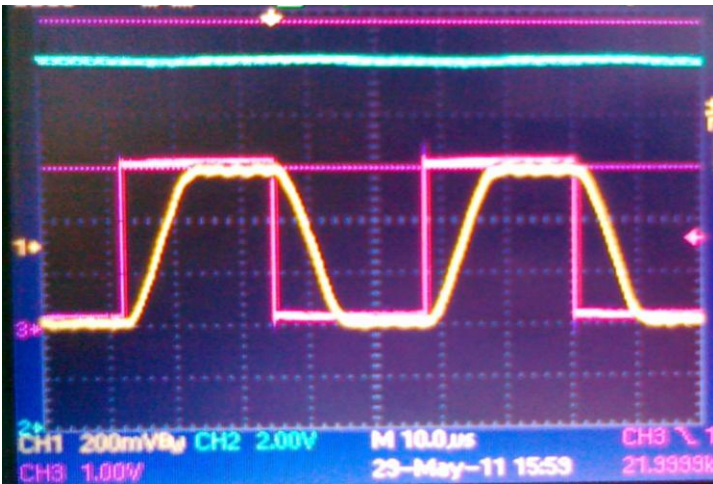
Figure.3 22KHz Tone Rising (7.5us) /Falling (7.5us) Edge
