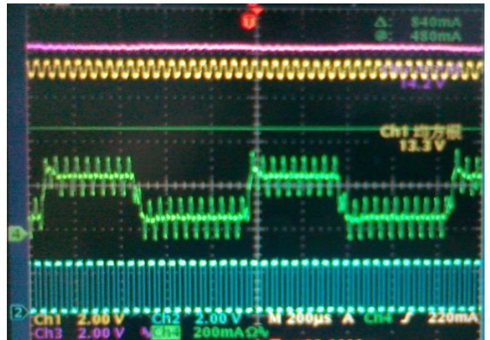
Figure.2 22KHz Tone ON 13.3Vout with Transient Loading (100mA → 400mA → 100mA, slew rate 255mA/7.5us)
