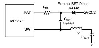
Figure 8—Add optional external bootstrap diode to enhance efficiency
