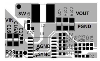
Figure 10—Recommneded buck converter layout
