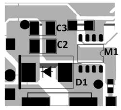
Figure 9—Recommended boost driver layout
