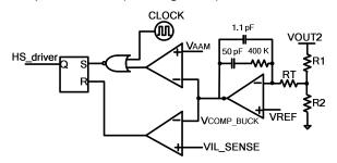
Figure 2—Simplified AAM control logic
