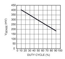
Figure 4—V<sub>SENSE</sub> vs. duty cycle
