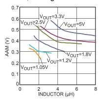
Figure 7—AAM selection for common output voltages (V<sub>IN2</sub> = 4.5 V - 24 V)
