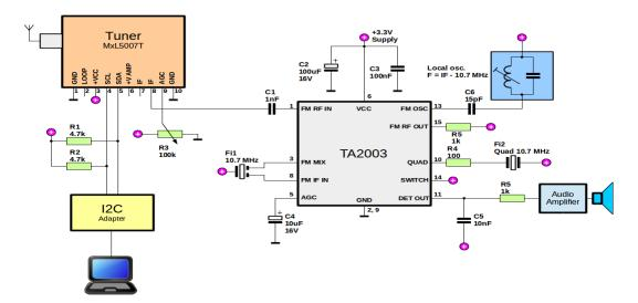
TA2003 FM detector for the tuner. Schematic based on datasheet and Uzzors2k webpage (CC-BY-NC-SA-3.0).
