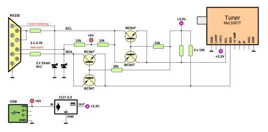
The adapter I built to connect the tuner to PC. Based on Claudio Lanconelli's SIProg and I2C level shifter from Arduino Playground.
