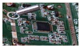
MxL5007T is a tuner IC designed mostly for digital signals (DVB-T, ATSC), but it can be used for analog reception too. It has a programmable IF output and it can receive anything from 44 to 885 MHz. There is no datasheet for it, but there are Linux drivers.
