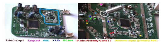
Left: the receiver PCB. The tuner is marked. Right: the IC connections and their meaning.
