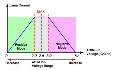
The negative input of error amplifier for current is IFB pin, and control loop is operated to make IFB level equal to ADIM level. The output of error amplifier for current, which is ICMP pin, is directly connected to main PWM generator.
