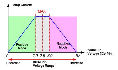
Burst PWM is generated using BDIM and triangular wave of CTB. The rising and falling slopes of BDIM operation are adjusted by capacitor which is connected between ICMP pin and GND. The source and sink currents of ICMP are 100uA. We recommend 300usec as rising and falling time.
