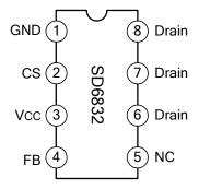
**Note:** it is recomended to connect pin 5 to pin Drain for better heat dissipation.
